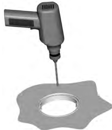
Fig. 5: Ring without Usable Screw Insert
